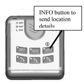
Press the INFO button to send a request with your current position to the Control Base.
